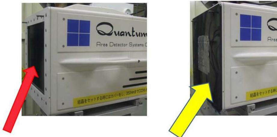
4. Please avoid hitting beam stopper, Co-axial camera and backing light accidentally. Before you can collect your data, please make sure that the beam stopper and back light at the right position. If the beam stopper is not at right position and **the direct beam will damage the CCD detector.**
